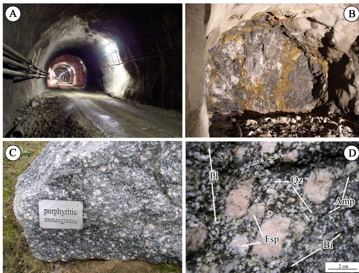
Figure 1. The geological environment of the Bataapati National Radioactive Waste Repository in Hungary. A) The underground subsurface gallery B) End of the tunnel under excavation C) A boulder of the examined monzogranite host rock D) Mineralogical assemblage of the porphyritic monzogranite lithotype.
