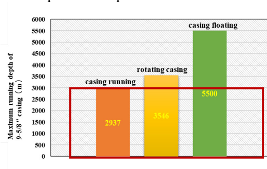
Figure 3. Maximum running depth of 9-5/8 " casing under different conditions-
