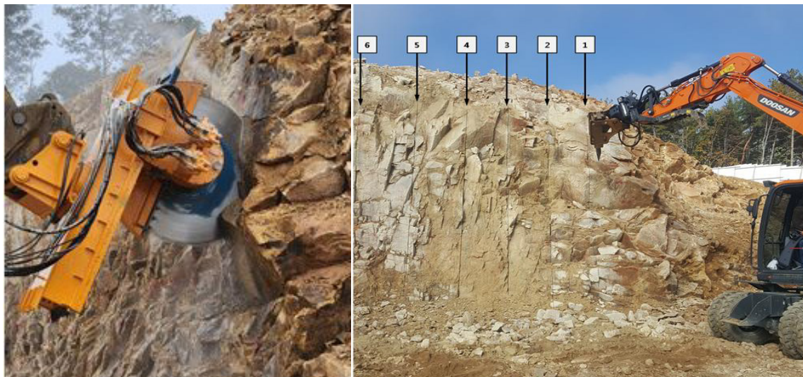
(a) Rock cutting by rocksaw prototype
