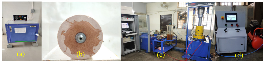
Figure 1. (a) Temperature furnace (b) Sandstone sampled glued to 20mm length cylindrical tube. (c) Rock triaxial setup (c) Hydro fracturing machine.
