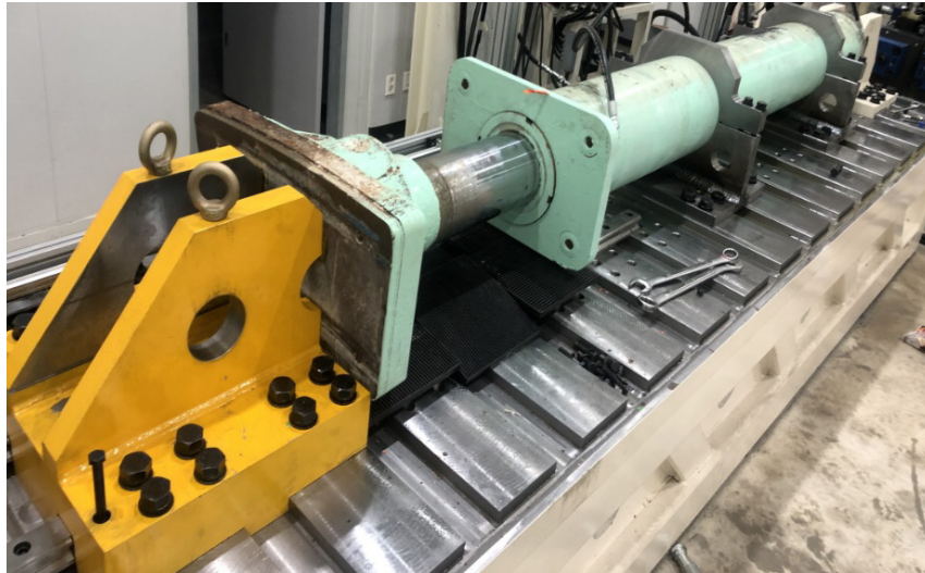
Figure 2. Testing equipment for thrust jack compression test.
