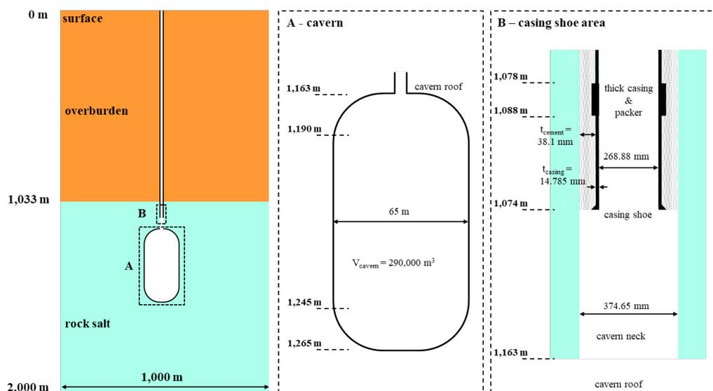
Figure 1. simulation model including cavern and wellbore.
