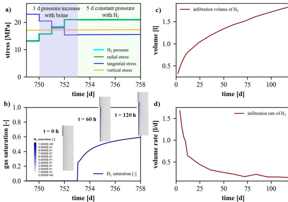
Figure 4. Hydraulic simulation during the mechanical integrity test, a) histories of stresses at borehole contour in a depth of 1,080 m, b) gas saturation at borehole contour in a depth of 1,080 m, c)  $H_2$  infiltration volume, d)  $H_2$  infiltration rate.
