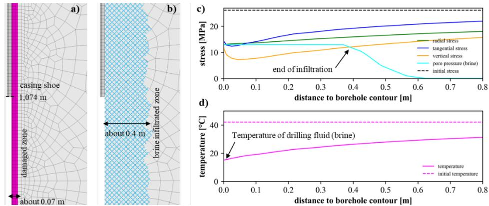
Figure 3. Borehole in the casing shoe area after drilling time  $t = 10$  d, a) damaged zone, b) brine infiltrated zone, c) profile of stresses in a depth of 1,075 m, d) profile of temperature in a depth of 1,075 m.
