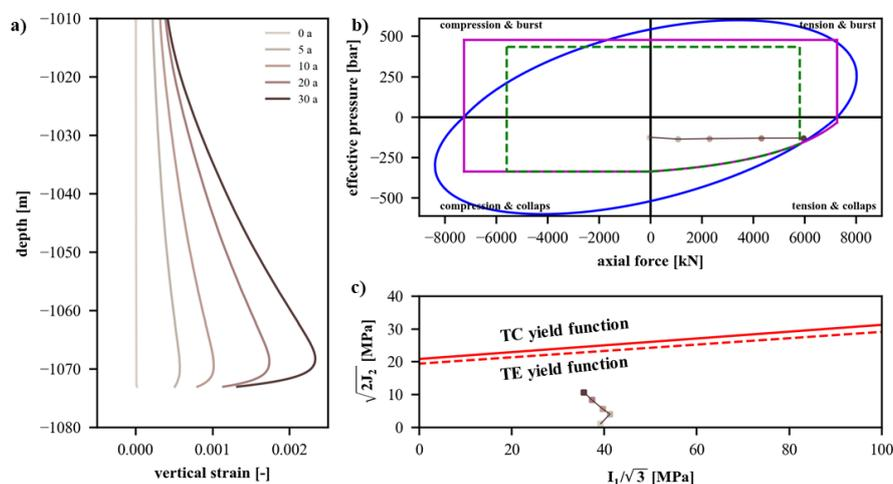
Figure 2. a) Profile of vertical strain along the casing over time, b) load of casing in a depth of 1,068 m using API standard, c) stress state of cement in a depth of 1,068 m.
