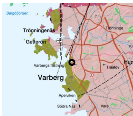
Figure 1. Bedrock map showing the Varberg area and the location of experiment (black circle). Main rock types: charnockite (green-brown) and gneiss – granitic, dioritic (pink), (Swedish Geological Survey 2023).
