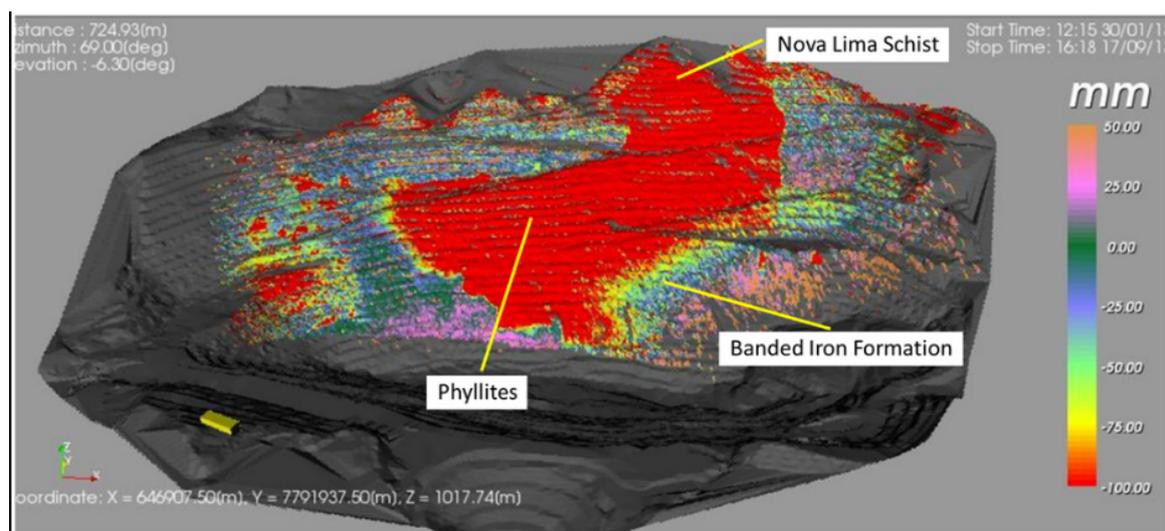
Figure 3. Interferometric radar result before compartmentalization and the main lithology associated with the shear zones.
