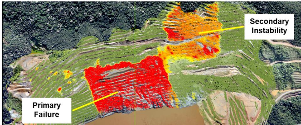
Figure 4. Interferometric radar result after geological compartmentalization showing Primary Failure and Secondary Instability.
