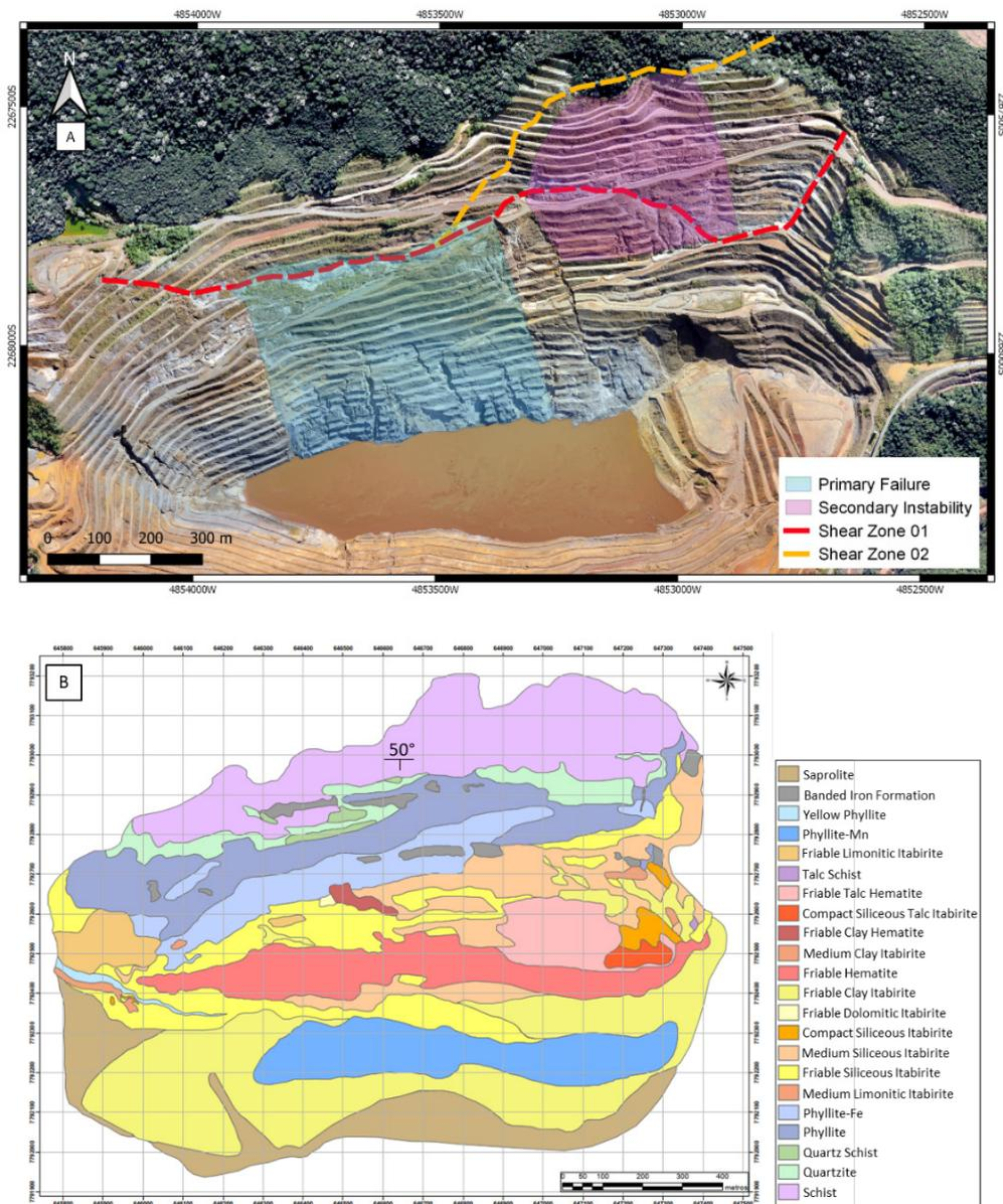
Figure 2. A- Main shear zones (Shear Zone 01 in red and Shear Zone 02 in orange). B- Gongo Soco Open Pit geological map, with medium dip direction around 50°.
