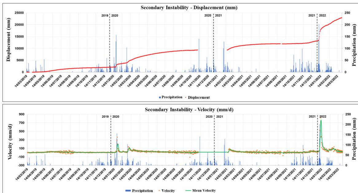
Figure 6. Secondary Instability's displacement, velocity and precipitation historical data.
