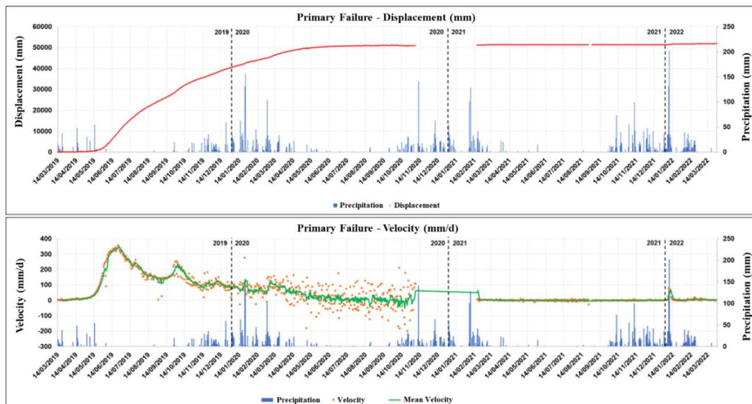
Figure 5. Primary Failure's displacement, velocity and precipitation historical data.
