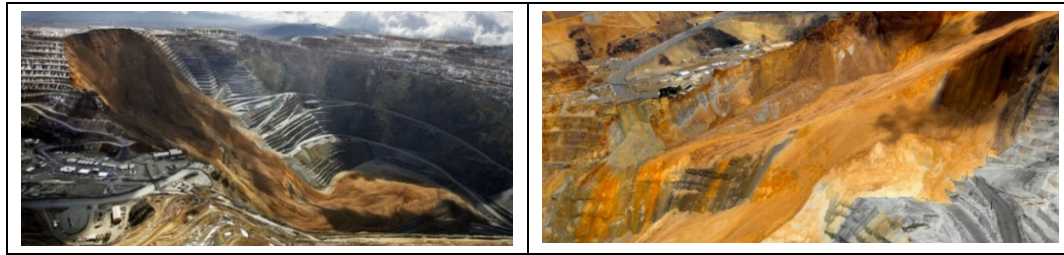
Figure 11. The massive Bingham Canyon mine open pit failure involved an adverse and unloaded ‘nose’ in its upper 1/3 rd and a major ½ km long fault surface in the upper region of the extraordinary 3km long failure path. Such failures can be understood by using up to four of the components of shear strength shown in Figure 12.
