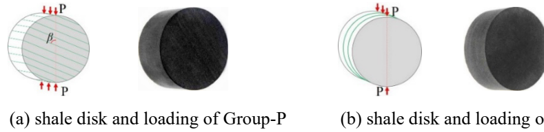
Figure 1. The groups of samples and loading diagram ( \beta is the angle between the loading and bedding).
