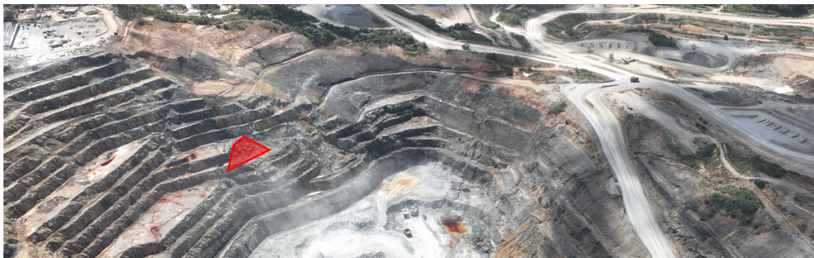
Figure 1. Aerial photograph of Moore Pit Pushback 15 looking South. Highly anisotropic Carbonaceous Sediments (UCS and LCS) in the upper (shallow) slopes, overlying various tuffs (FDT and QBT). Red polygon indicates the location of the actual failure.
