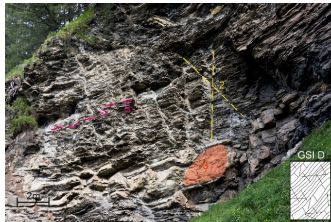
Figure 2. Outcrop, representative for strongly folded and jointed rock mass of Bündner Schists in the valley of Vals: S—schistosity (magenta), 2—conjugate discontinuities (yellow), 3—fault plane (red).
