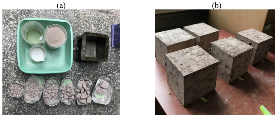
Figure 1. (a) Constituents of artificial bimrock samples, (b) artificial cubical bimrock samples drying at room temperature.
