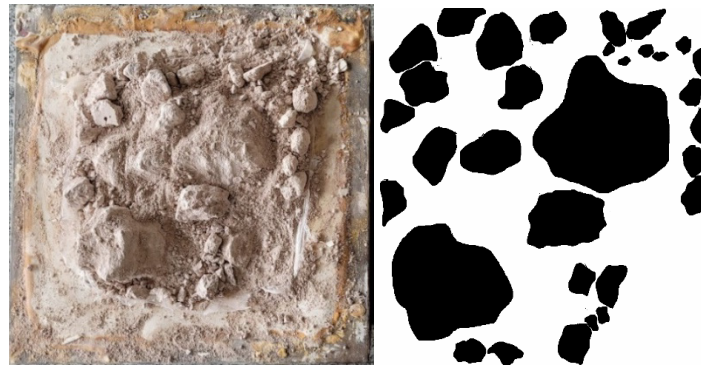
Figure 6. The failure surface and digitized image of sample no. 11 (VBP= 40%, VBPf s =42%).
