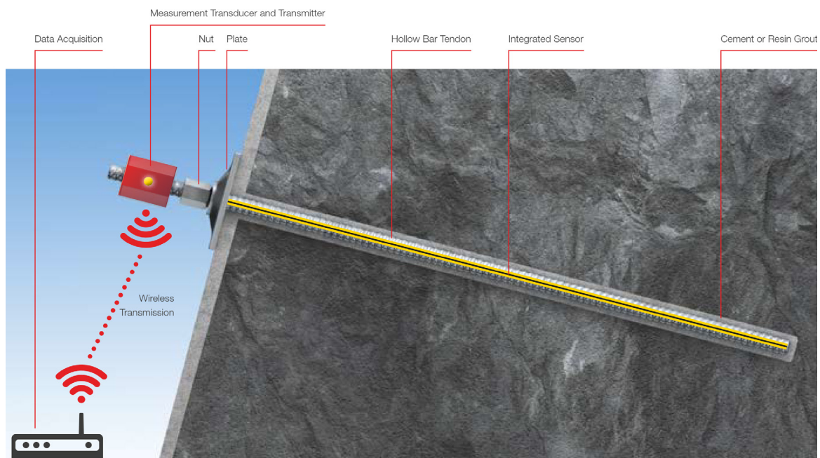
Figure 1. low-cost intelligent rock bolt assembly.
