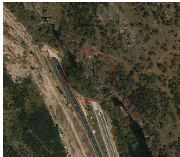
Figure 2. Upper view of the site. Red circles show the large fractures that separate the columns from the cliff.
