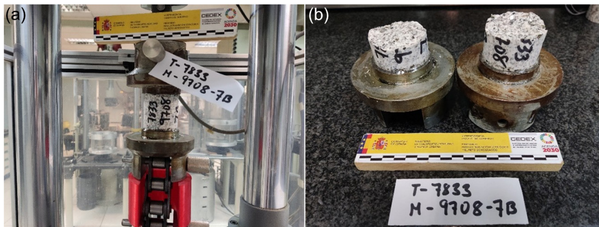
Figure 3. (a) Specimen (H/D = 1) mounted in the loading frame prior to testing; (b) Same specimen after a valid test.
