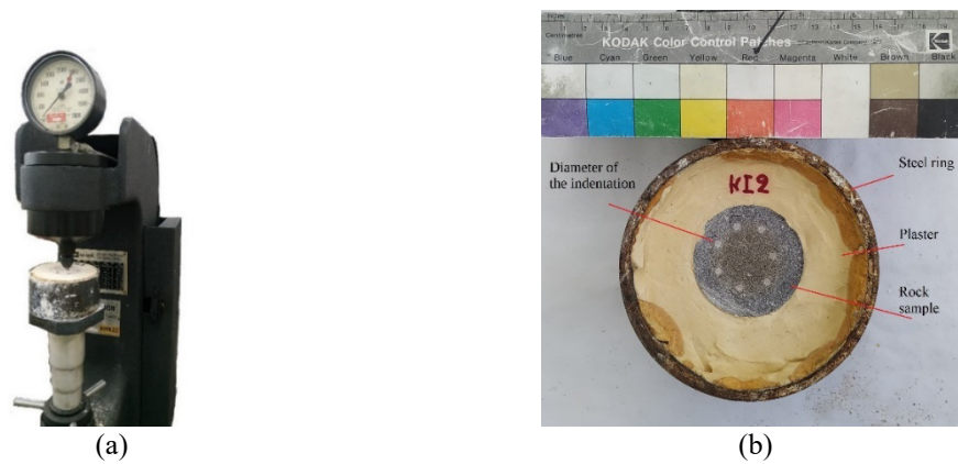
Figure 1. Photographs of the Brinell hardness tester used (a) and a rock specimen cast in a steel ring using dental plaster. Note the number and size of the indentations (b).
