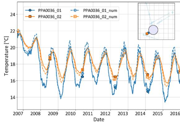
Figure 3. Measurements and numerical results of the temperature evolution in the rock (near field) at SMGR3 section (-479 m).
