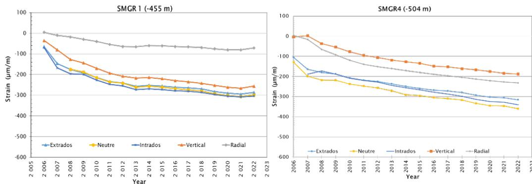
Figure 6. Evolution of the annual average strain measured with the vibrating-wires in SMGR1 and SMGR4.
