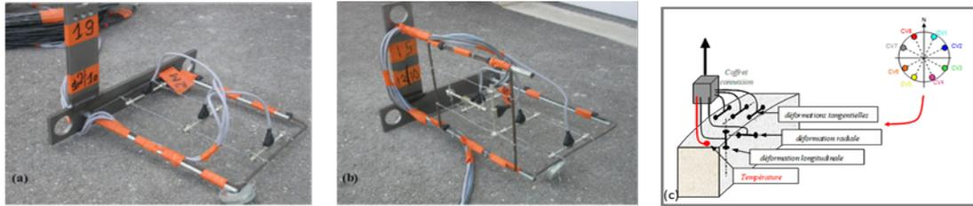
Figure 5. Position of the vibrating-wires and temperature sensors in the instrumented sections of the shaft's lining.
