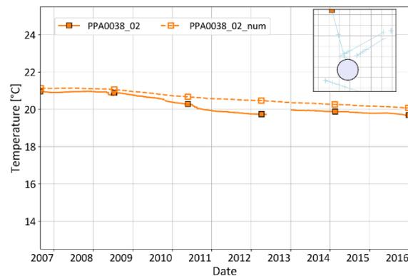
Figure 4. Measurements and numerical results of the temperature evolution in the rock (far field) at SMGR3 section (-479 m).
