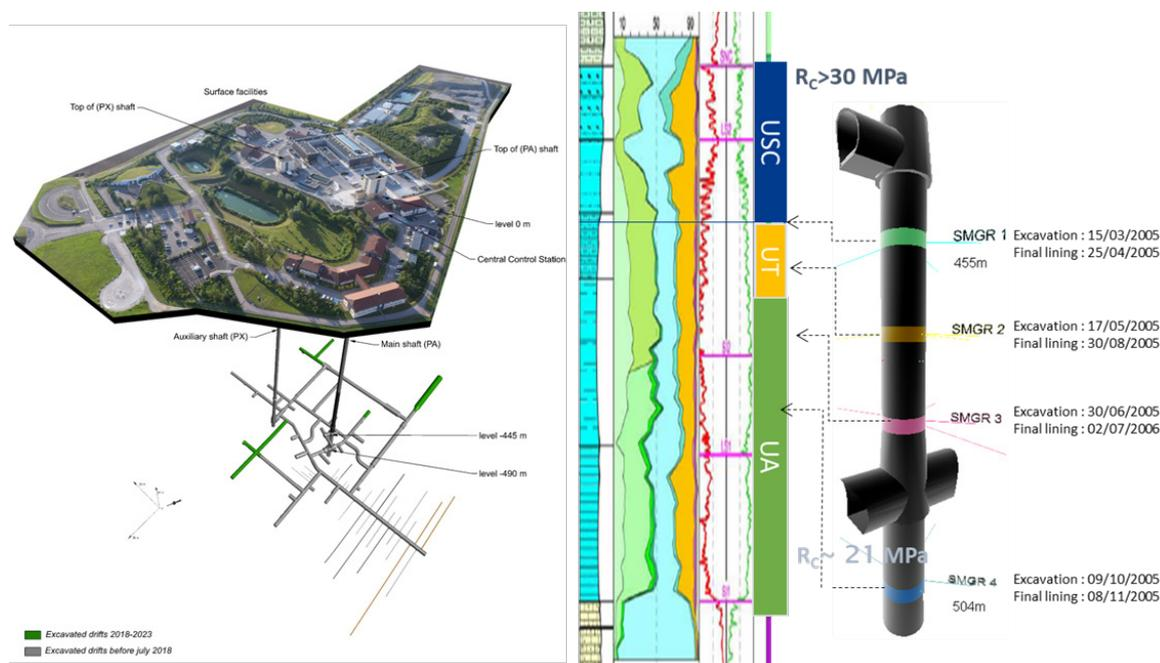
Figure 1. Representation of the MHM URL (left), and the position and clue dates of SMGR sections in homogeneous geological units of the COx claystone (right).
