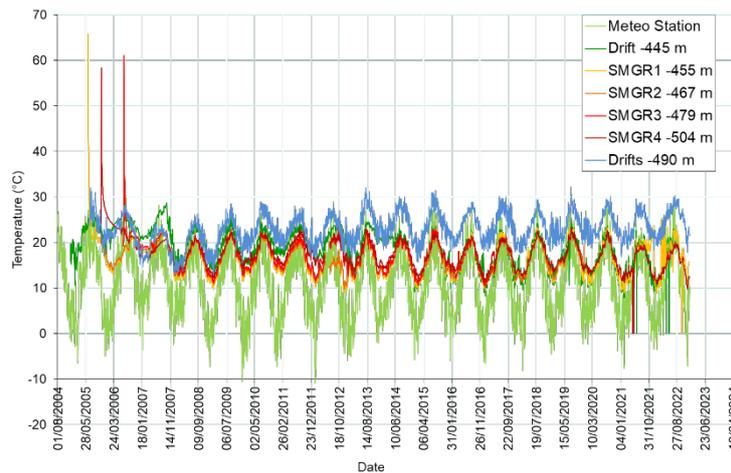
Figure 2. Seasonal variation in temperature in the shaft, in the -445 m drifts, in the -490 m drifts and in the surface weather station.
