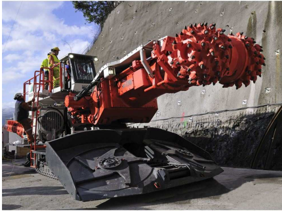
(a) Photograph of 130 ton Roadheader
