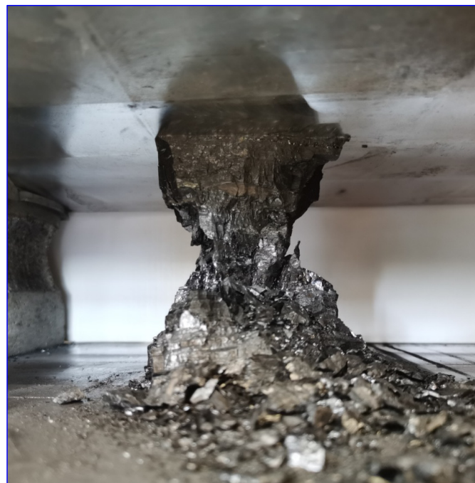
Figure 5. Final failure pattern of the coal pillar after catastrophic bursting failure.
