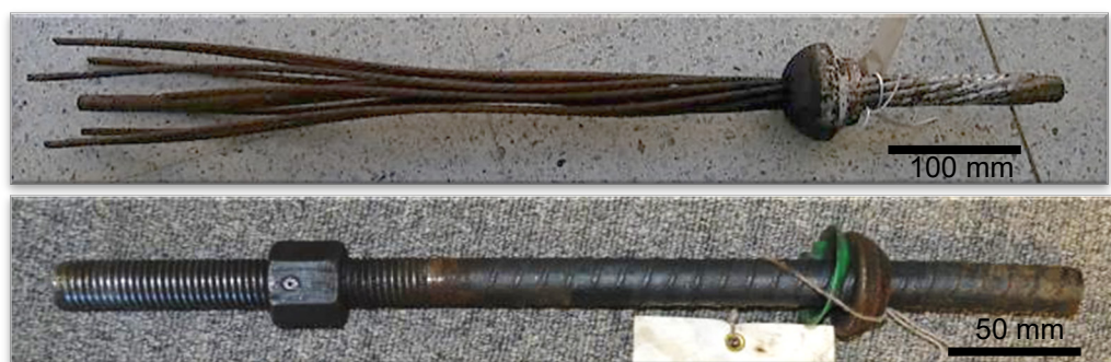
Figure 1. Fractured cable bolt (above) and rockbolt (below) due to HISCC from the mines.
