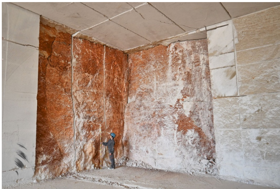
Figure 1. Typical example of discontinuities in thick-bedded and karstified limestone deposits.
