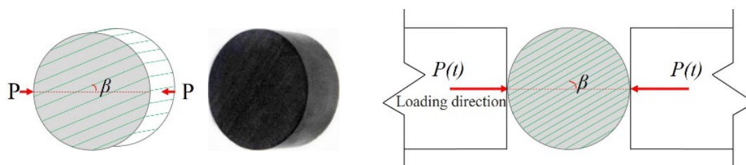
Figure 1. The samples and loading diagram ( \beta is the angle between loading direction and bedding).
