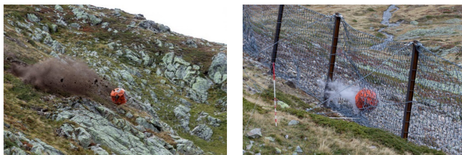
Figure 2. Left: A test block, released by helicopter bounces, rolls and slides down the slope. Right: Fully instrumented flexible rockfall protection barrier experiencing a random rock impact.
