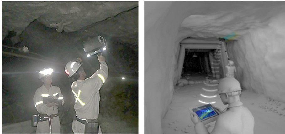
Figure 4. Left: Illustration of the physical use of the GPR, rolling it along the hangingwall. Right: Illustration of how to operate the GPR in an underground environment to detect the geologic structures in the hangingwall, shown in real time on the tablet. It is used to gain a better understanding of the presence of structures that may lead to instabilities.
