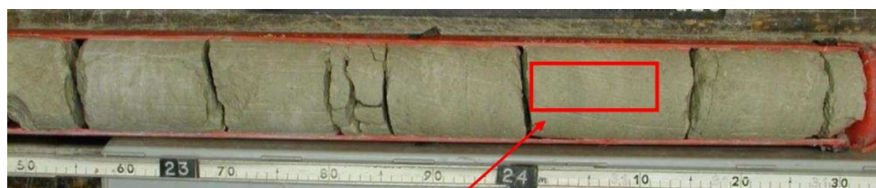
Figure 1. Core photo of Copenhagen limestone from Cityringen project (SGI, 2012).
